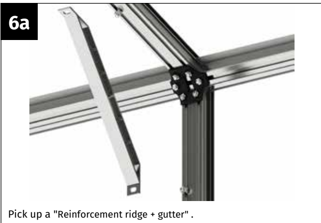
Align the M6x12 mm screws so that the stiffener can be fitted and put it in place.
