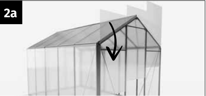
2a Insert the twin-wall sheets from above into the shaped "U" of the side corner profiles and the back wall braces. It may be necessary to loosen the wind bracing again on the inside to be able to align the greenhouse exactly plumb.
