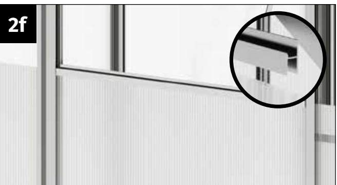
2f Place an H-profile on each of the three twin-wall sheets of the back wall. See also the detailed picture of how to attach the H-profiles!
