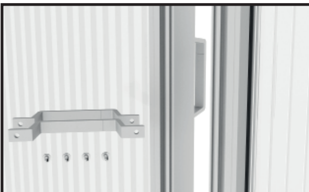
Assemble the door handles on the inside of the greenhouse in the same way.
